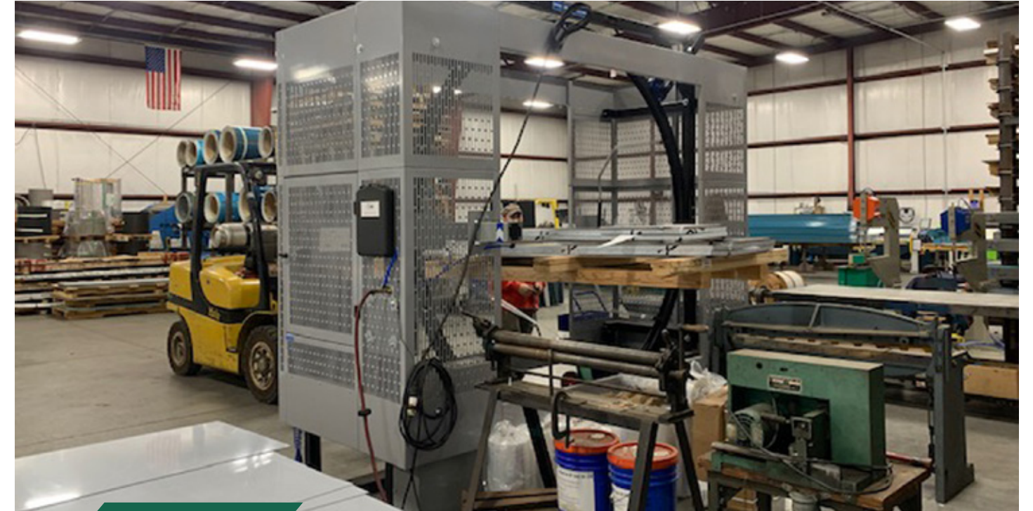
A TAB Wrapper Tornado orbital wrapper applies stretch wrap 360 degrees around and under a pallet load of metal building products at Penn Sheet Metal.
