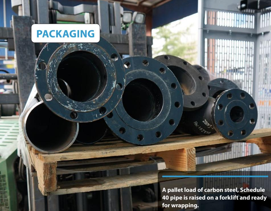
A pallet load of carbon steel, Schedule 40 pipe is raised on a forklift and ready for wrapping.
