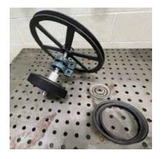
Complete system with fly wheel, bearing belt and V idler preassembled with shaft, two pillow block bearings and key ways.
