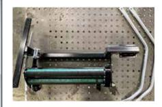
Stretch film roll dispensing unit arrives pre-assembled with the arm, rollers, and other components. Interchangeable for Dual Dispensing machines.
