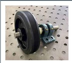
Wheel with shaft and two pillow block bearings arrives preassembled. Rubber tread wear indicates need for replacement.
