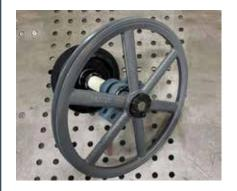
Fly wheel, bearing belt and V idler pre-assembled. Look for wear on the rubber tread before it detaches from the hub, keep two on hand. Typical service life of 5 years.
